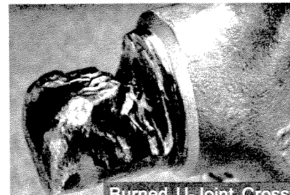
Burned U-Joint Cross
